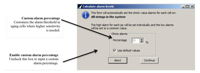
All alarms for all battery strings will be programmed at the calculated level, using the selected percentage above the current measured ohmic reading. Once the alarms have been set a dialog will appear informing the user that the alarm levels will be automatically recalculated in 35 days' time (right).
