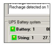
be recorded during the recharge period. The software will indicate the recharge event with a small recharge icon in the battery and string tab.
