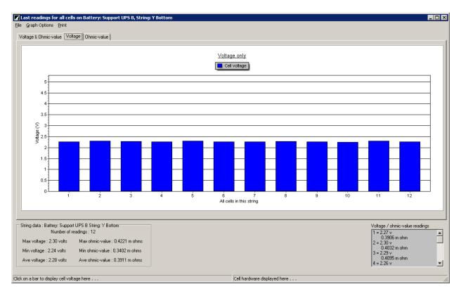
This is a typical string voltage graph and shows an average voltage of 13.47 volts – a per cell value of 2.25 volts. Manufacturers such as C&D Technology recommend a low voltage limit of 2.16 volts per cell or 4% drop in voltage. Therefore selecting a voltage level of 4% below this average voltage (12.93V) would provide good voltage alarm sensitivity while not presently causing an alarm trigger (in the above example the present lowest voltage is shown as 13.11v).
