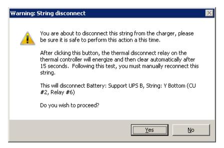
Selecting "No" will cancel the test, while selecting "Yes" will proceed to activate the displayed relay attempting to remove the string from operation. Cellwatch will indicate that the string has been disconnected and ask the user to clear the relay and 're-arm' Cellwatch in the alerts window. Before proceeding verify that the string was taken offline and that Cellwatch was connected properly to the circuit that removed the string from operation.
