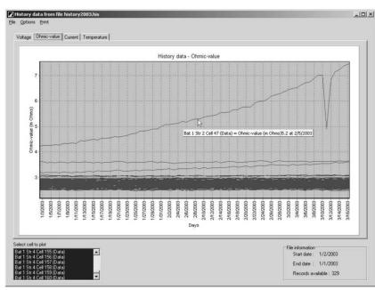
significant improvement in the ohmic value of the bloc. However, as can be clearly illustrated, the trend always reverts back to an upwards trend.
