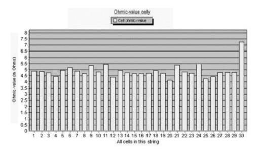
The 'Automatic Ohmic Alarm Setting' feature sets individual jar alarm settings automatically. It can be run across the entire system, or may be utilized on a string-by-string basis.
