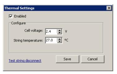
Using the 'Test string disconnect' allows users to verify that the relay circuit is configured correctly to remove a string from operation. Once activated, the relay tied to this physical string will be activated for 15 seconds. If configured properly to an external breaker, the string should be taken offline until manually reconnected. To proceed with the test feature a password must be entered and the
