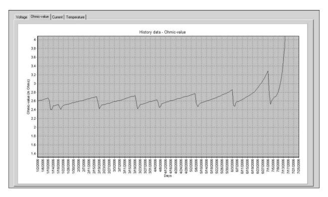
In the example shown above, failure of the jar can be predicted one month or more before failure by observation of both the slope of the ohmic value increase and by the high level the ohmic value reached just before the recharge cycle started.
