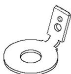
Connection to the battery is made using  $\frac{1}{4}$  inch fast-on terminals to tab washers supplied as part of the system. These tab washers are fitted directly to the battery posts or on to the inter cell straps. For a visualization of the connection of a DCM to a battery see the diagram below. Tab washer sizes vary from M5 (1/5 in.) to M12 (1/2 in.).
