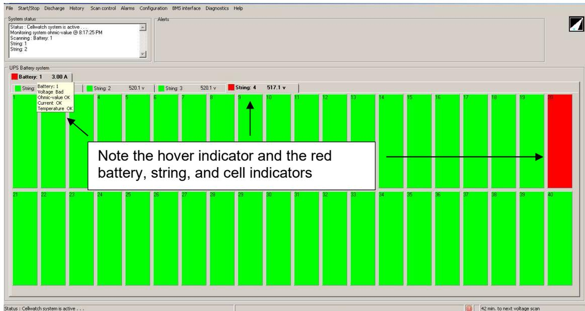
It is highly recommended to have a permanent monitor setup connected to your iBMU. A KVM switch is recommended if more than one iBMU are utilized due to the size of the installation. Alternately, some users establish a remote connection into the system allowing battery status information to be visible outside of the battery room or remotely from the site itself.
