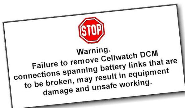
This unit must be disconnected **prior** to separation and subsequent removal of the link. (Please note each unit in this system spans many mono-blocs)
