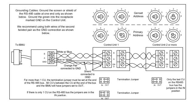
Note: Connect the stranded drain wire wrapped around the other wires of the Belden cable into the GND connection. Connect in the first CU connector only to ensure best protection from radiated noise. Do not land the drain on both sides of any RS485 wiring section, (iBMU to CU) or (CU to CU).
