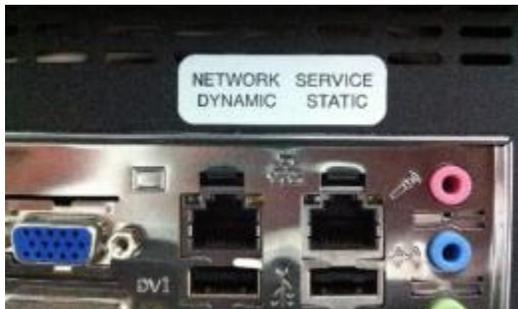
Cellwatch is designed to be remotely accessible in order to streamline the interactions with the software and simplify the retrieval of battery data. There are several hardware and software options for interfacing with the iBMU. The most common method is using a keyboard, monitor, and mouse and the primary alternative is Windows Remote Desktop.
